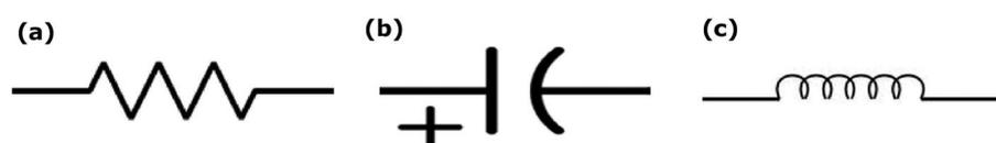
**Figure 7.** Basic electrical circuits for electrochemical impedance spectroscopy (EIS): (a) resistor ( $Z = R$  (Ohms),  $0^{\circ}$  phase shift), (b) capacitor ( $Z = -j/\omega C$  (Farads),  $-90^{\circ}$  phase shift) and (c) inductor ( $Z = j\omega L$  (Henrys),  $90^{\circ}$  phase shift) (authors original image).
