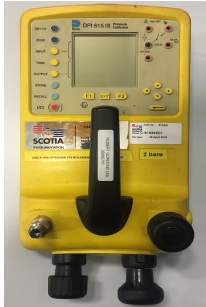
Figure B.1: Druck pressure calibrator
