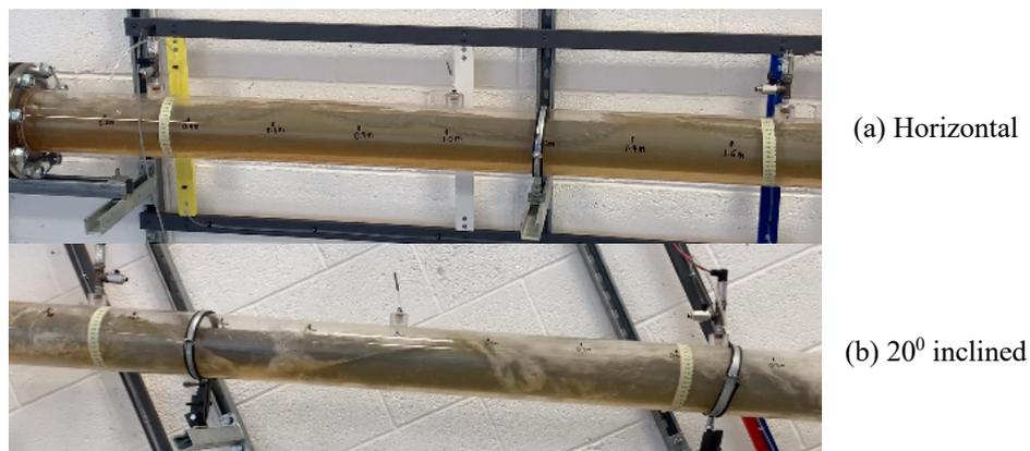
Figure 7.20: Comparison of the fluid distribution and mixture properties of slug flow in the horizontal and inclined annuli test sections
