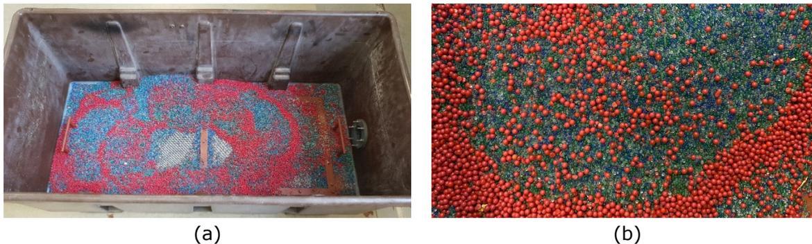
Figure 3.3: (a) solids separation tank and (b) glass and plastic beads
