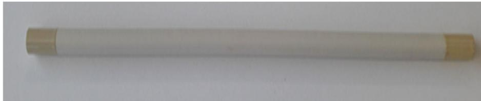
Figure 6: Picture of 15nm (25mm OD) membrane
