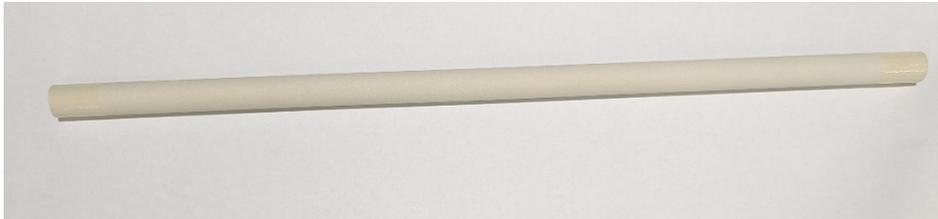
Figure 7: Picture of 200nm (10mm OD) membrane
