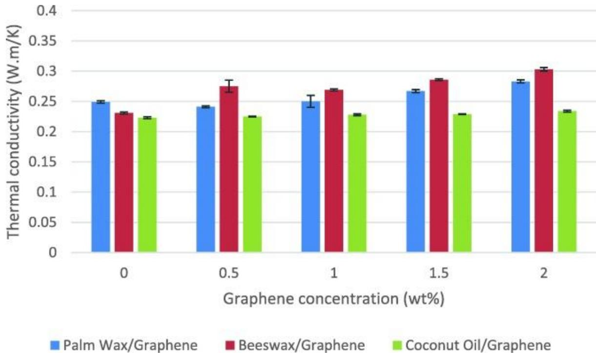
Fig. 5. Experimental thermal conductivity of BPCMs/Graphene.
