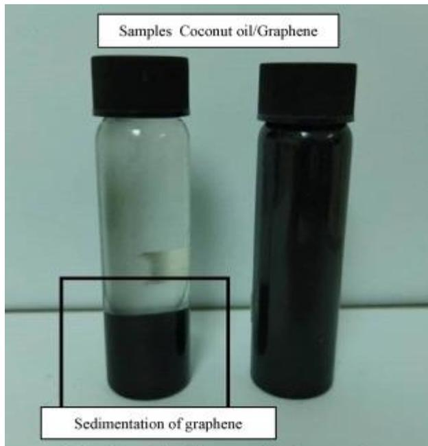
Fig. 6. Observation of coconut oil/graphene sample
