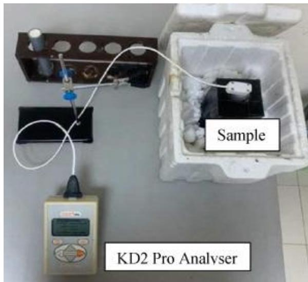
Fig. 3. Thermal conductivity measurement using KD2 Pro Analyser.
