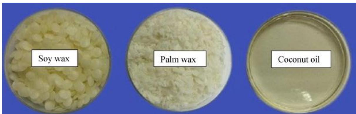
Fig. 1. Pure biobased phase change materials (BPCMs).
