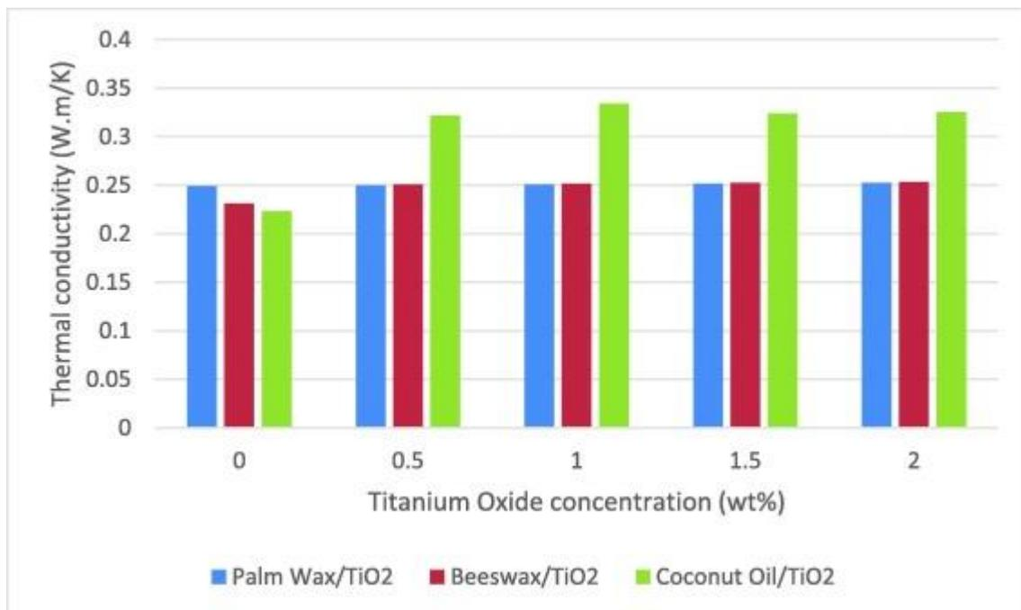
Fig. 7. Theoretical thermal conductivity of BPCMs/Titanium Oxide as calculated from Maxwell Garnet equation.
