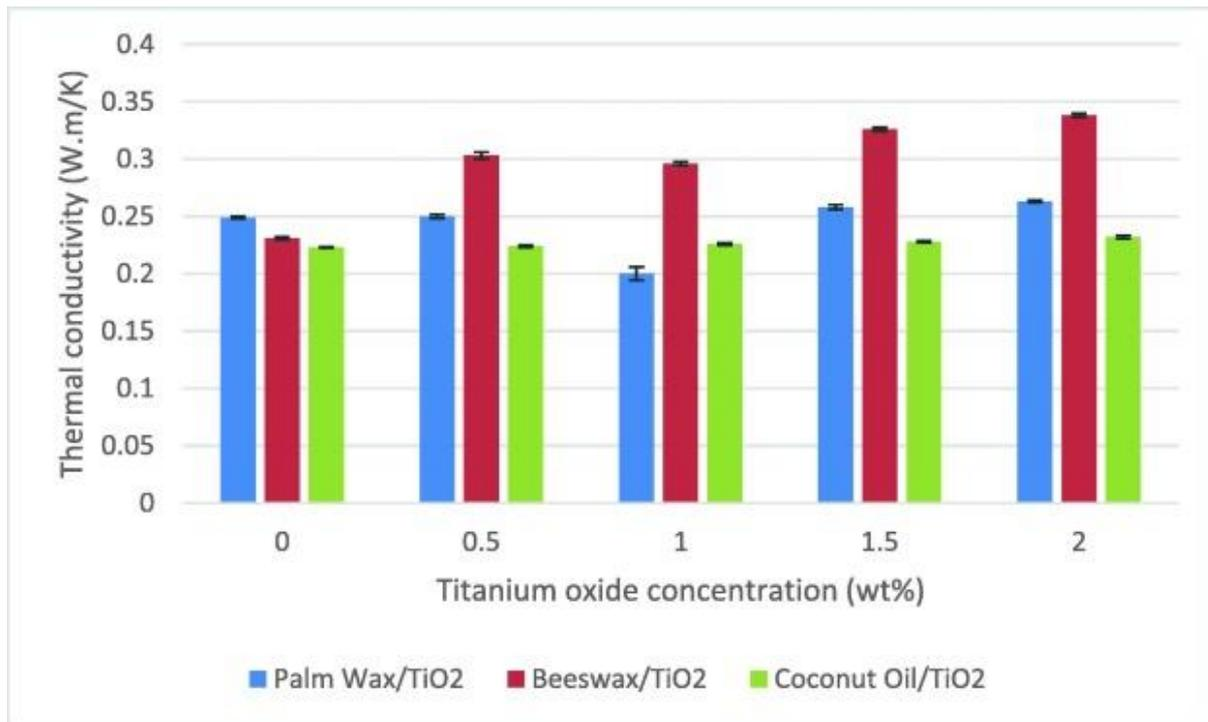
Fig. 8. Experimental thermal conductivity of BPCMs/Titanium Oxide.
