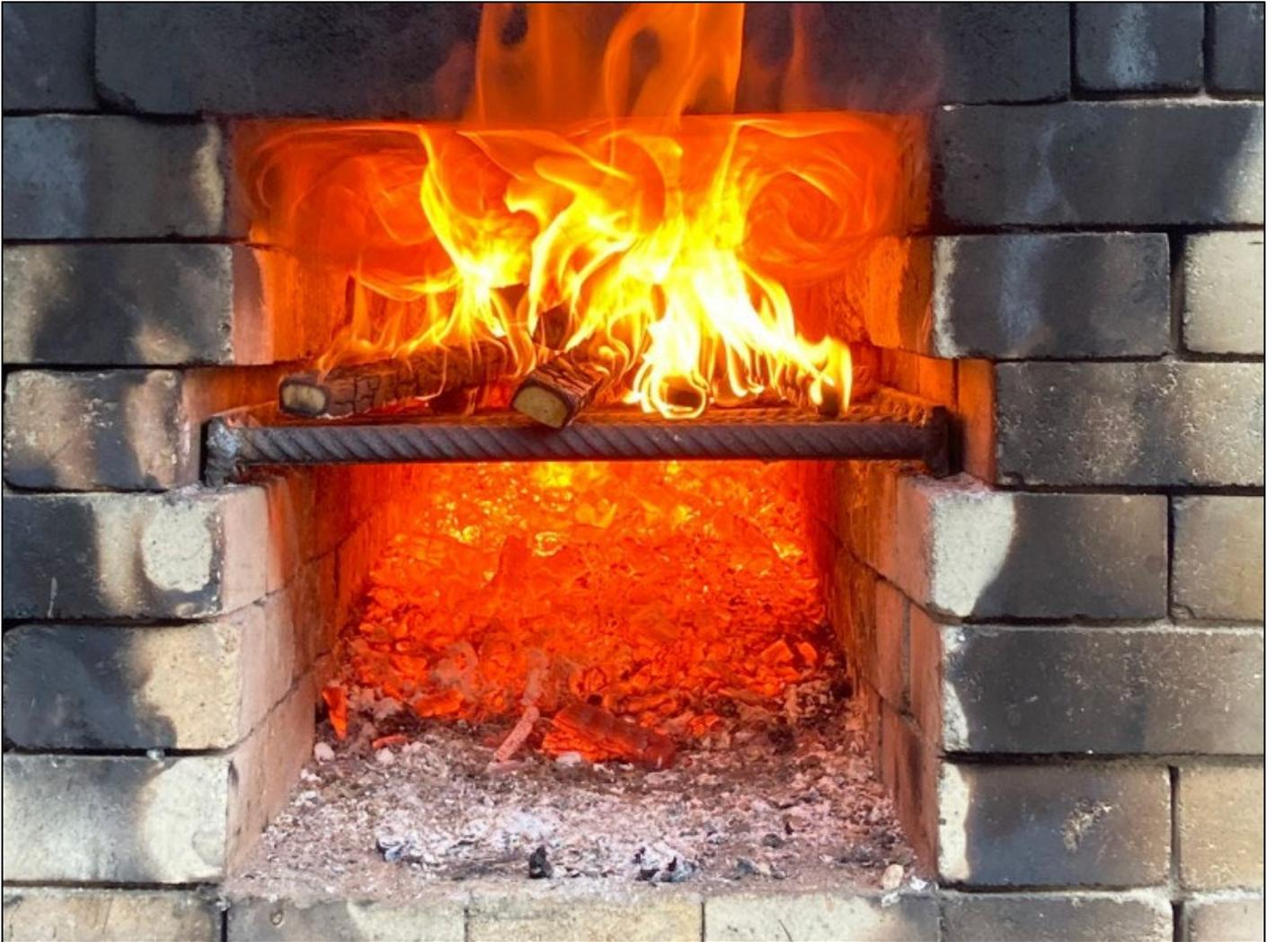
Figure 1. Photograph of a wood-fired kiln.
