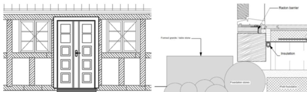
Figure 4. Front door and detail with large formed granite / table stone. Drawings with permission from ISAGER Architects, Odense, Denmark
