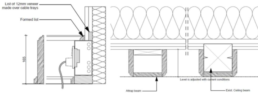
Figure 7. Sockets and other technical outlets and substitution beam. Drawings with permission from ISAGER Architects, Odense, Denmark
