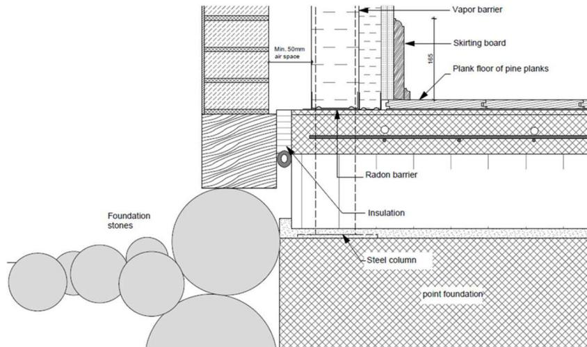
Figure 3. Detail with stone foundation
