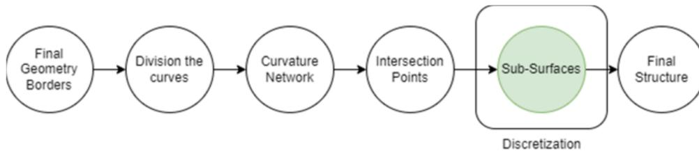
Figure 3 Curvature Network Parametric Logic, Credit by Erfan Zamani
