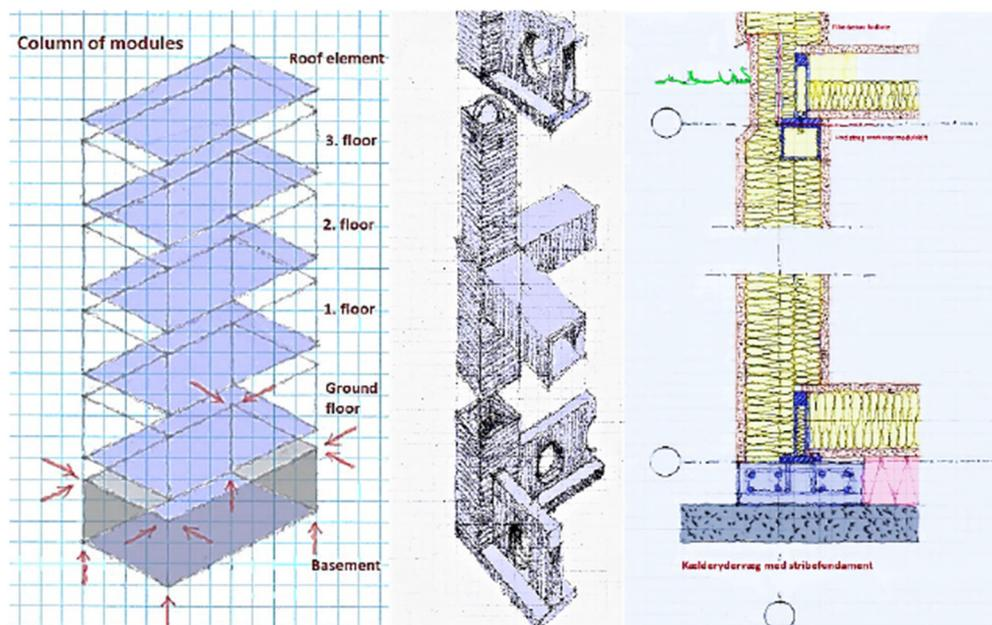
*Figure 10: Columns of modules, load bearing parts, and standard construction.*
