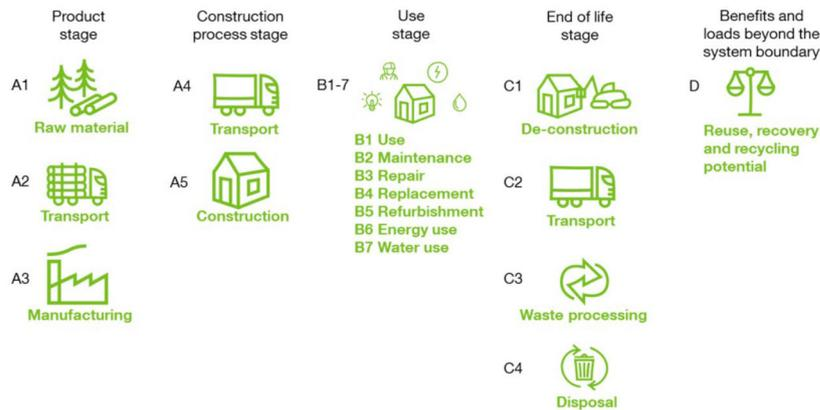
Figure 7.0. Embodied Carbon Over Life Cycle (Stora Enso 2020).
