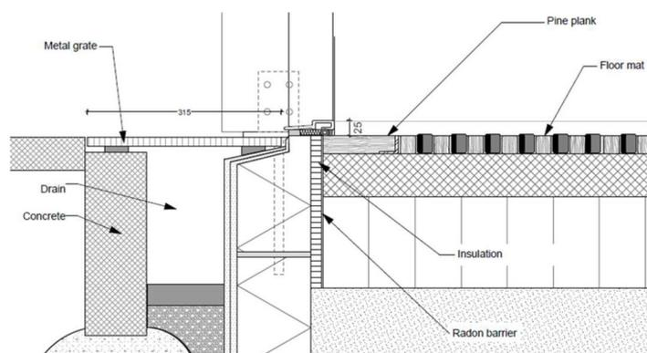
Figure 5. Entrance with level-free access. Drawings with permission from ISAGER Architects, Odense, Denmark
