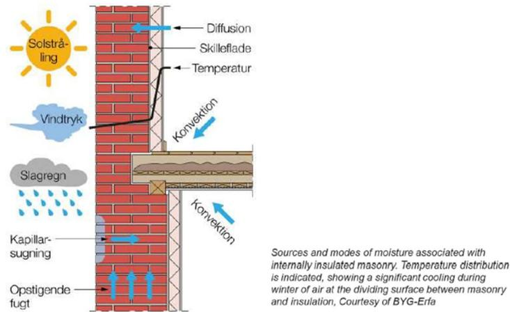
Figure 2. Sources and modes moisture associated with internally insulated masonry
