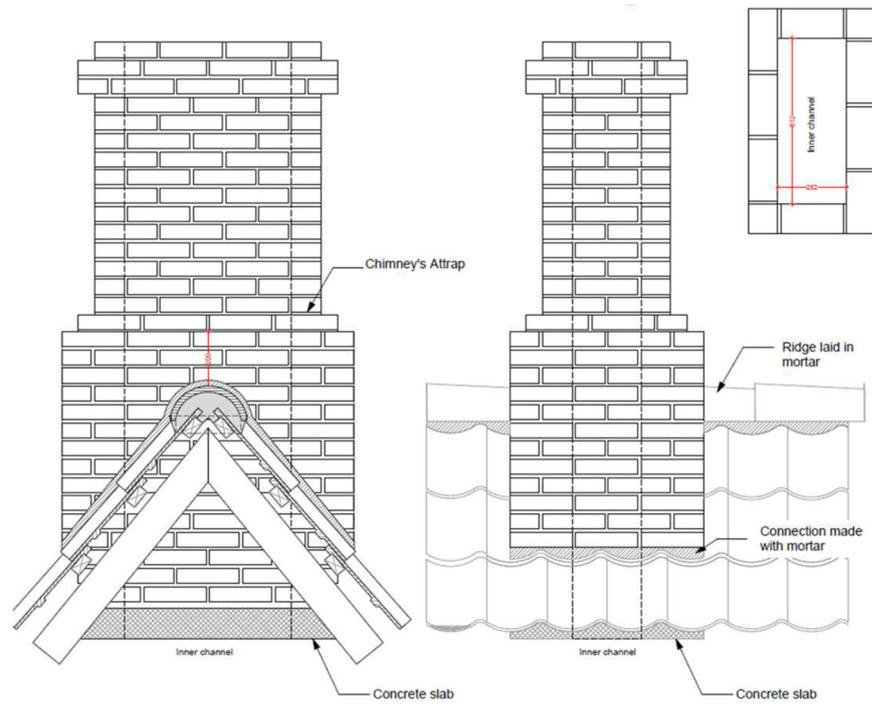
Figure 6. Chimney substitution. Drawings with permission from ISAGER Architects, Odense, Denmark
