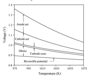
Higher temperature leads to better performance due to reduction in anode and cathode activation overpotential. However, it creates thermal stress and less durable cells
