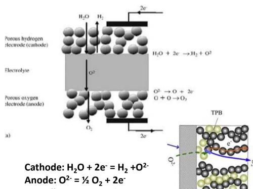
а **▶** Interconnection → Anode ► Electrolyte Cathode Steam Flow in
