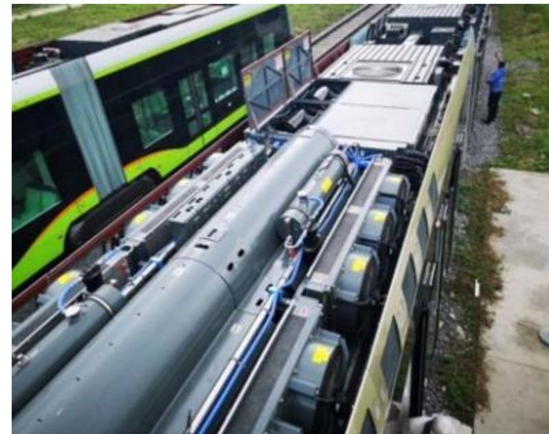
Hydrogen tank and Ballard fuel cell system on CRRC-Sifang light rail
