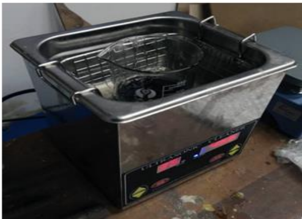
Fig. 1. Sonication of 1 wt% graphene in epoxy resin using bath sonicator.
