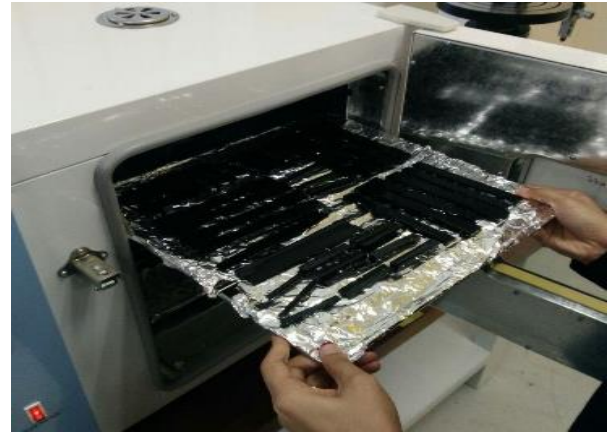
Fig. 2. Post curing of samples at 150 ^{\circ}\text{C} in a drying oven.
