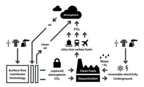
**Figure 12.** Direct air capture using  $CO_2$ -affinity ceramic membrane technology (um-DAC®).
