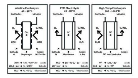
**Figure 3.** Workings of the three types of electrolysers (*from left to right*): alkaline (AEL); acidic (polymer electrolyte membrane); and solid oxide electrolyser cells (SOECs).
