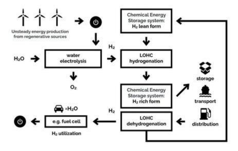
Figure 9. Liquid organic hydrogen carrier technology.
