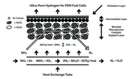
**Figure 8.** Combined ammonia cracking with ultra-pure  $H_2$  production in a catalytic membrane reactor with a heat-exchange jacket (CMR-HEJ<sup>®</sup>).
