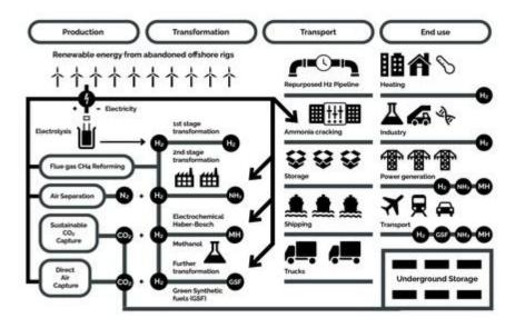
**Figure 1.** Future zero-carbon H<sub>2</sub> infrastructure chain.
