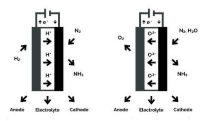
**Figure 6.** Diagrammatic illustration of solid-state electrochemical ammonia synthesis – proton-conducting membrane electrolyte (*left*); and oxide-ion membrane electrolyte (*right*).
