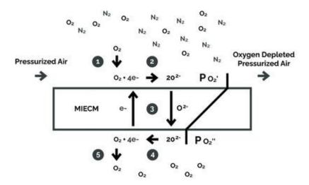
**Figure 5.** Schematic representation of the four-step oxygen transport process through a mixed ionic electronic ceramic membrane (MIECM), with different oxygen partial pressure  $(PO_2' > PO_2'')$  on both sides.
