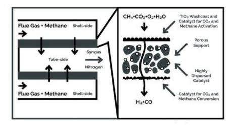
**Figure 14.** Forced flow-through catalytic membrane reactor showing reactor operating configuration (*left*) and enlarged view of the membrane surface and cross-section, revealing nano-dispersed catalysts and pathway of reactants to generate syngas (*right*).
