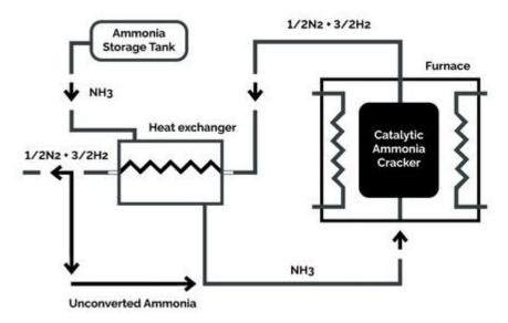
**Figure 7.** The principal flow scheme of a conventional ammonia cracker.
