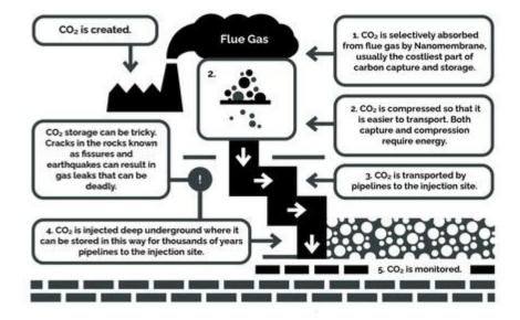
Figure 11. Traditional membrane carbon capture technology and sequestration.
