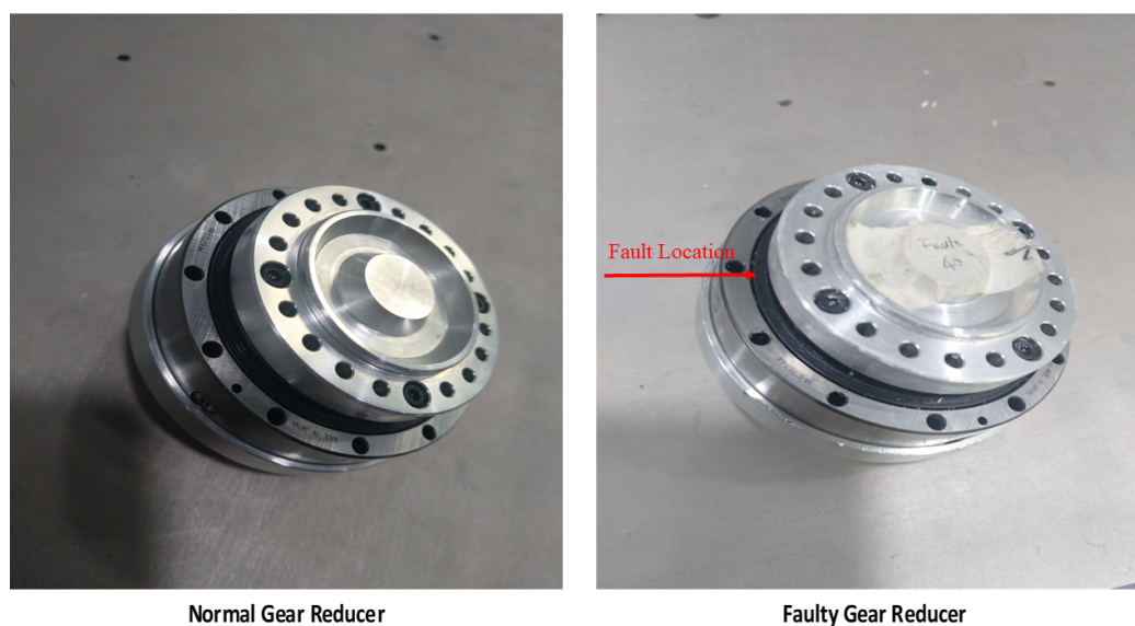
Figure 6. Strain wave gear reducer for Robostar Axis 3: normal and faulty.
