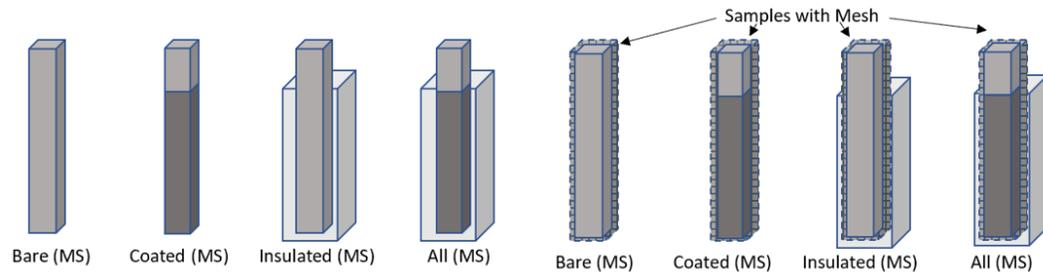
Figure 6 – No Mesh and Mesh Samples
