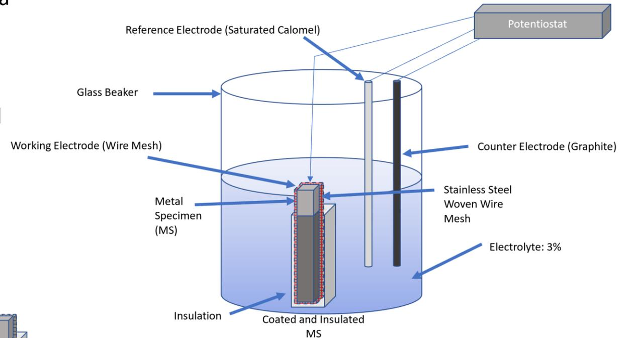
Figure 5 – Experimental Setup with Sample
