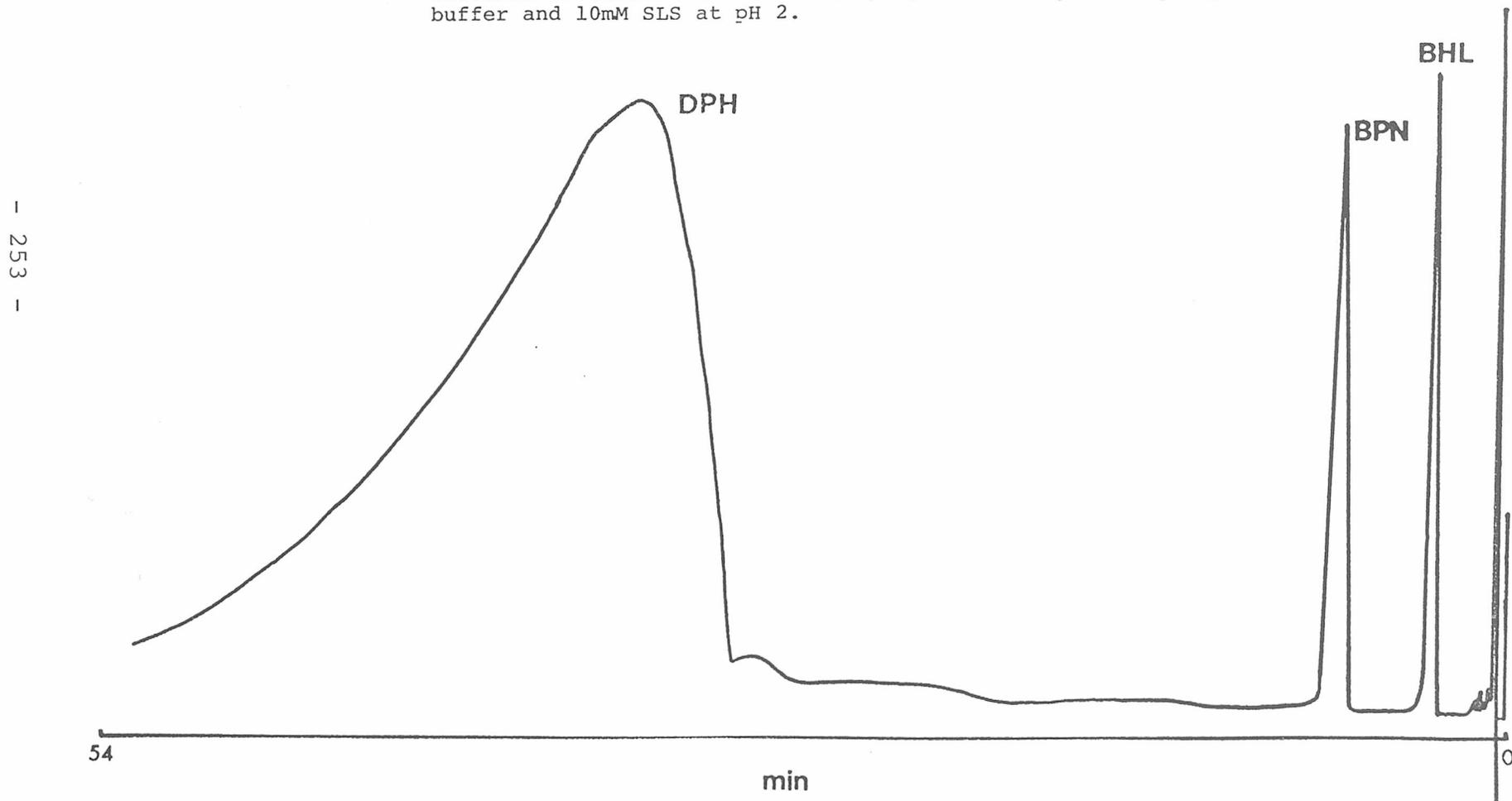
Figure 8.5 Showing the separation of DPH and its decomposition products using a 4.6x50mm column at 0.5AU. Solvent: acetonitrile : water (30/70) containing 120mM phosphate buffer, 10mM SLS and 5mM TBA at pH 2.
