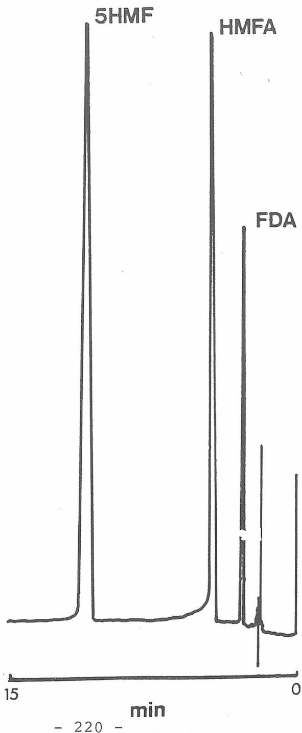
Figure 7.2 Showing the separation of 5HMF, HMFA and FDA at 0.2AU. Solvent: water containing 10mM phosphate buffer and 8mM TBA at pH 7.
