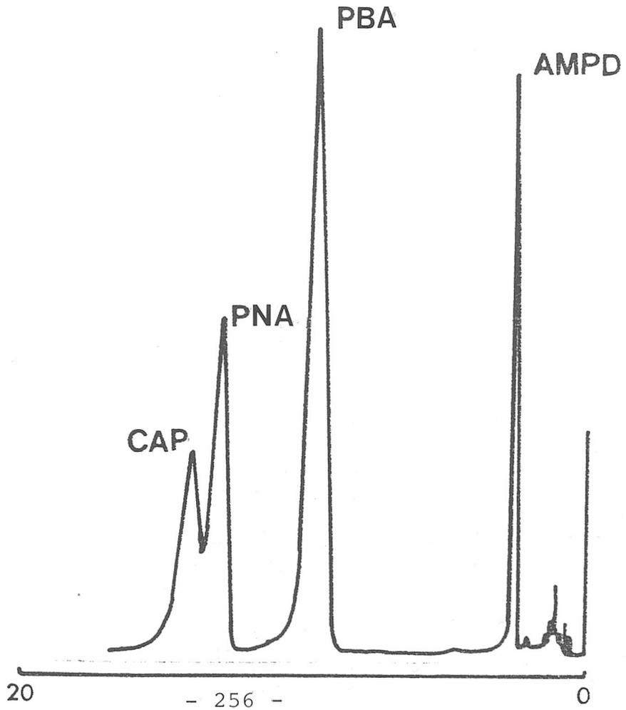
Figure 8.8 Showing an optimum specimen chromatogram for the separation of CAP and its decomposition products using a 4.6x200mm column at 0.2AU.
