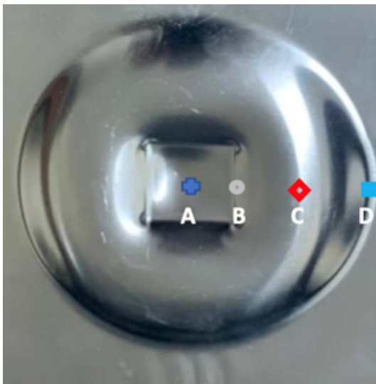
Figure 12. Velocity profile investigated at four points on the deformed Al 6061-T6 sheet.
