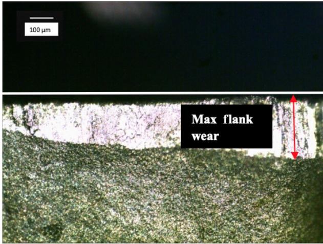
**Figure 3.** Optical microscopy image showing maximum flank wear.
