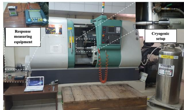
**Figure 2.** CNC Turning centre with cryogenic setup and response measuring equipment.**Table 2.** Chemical Composition (wt %) of Ti-6Al-4V.
