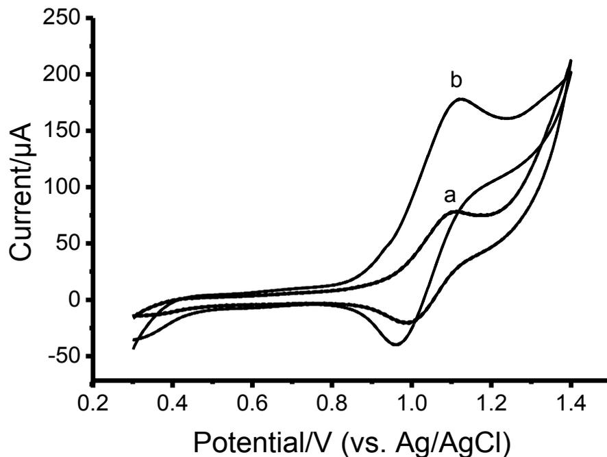
**Figure 3.** Cyclic voltammograms of the glassy carbon electrode. (a) 1 mM  $[\text{Ru}(\text{bpy})_3]^{2+}$  in acetate buffer pH 4; (b) 2000ng/mL of Flunitrazepam in 1 mM  $[\text{Ru}(\text{bpy})_3]^{2+}$  with 1 mM acetate buffer at pH 4 both acquired at scan rate 100 mV/s.
