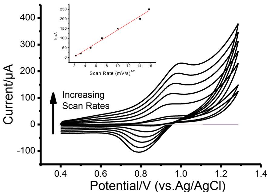
**Figure 4.** Voltammograms for scan rates between 5 and 250 V/s in a solution of 2000 ng/mL Flunitrazepam, 1 mM  $[\text{Ru}(\text{bpy})_3]^{2+}$  with 1 mM acetate buffer at pH 4. The cross-lines indicate the point of origin and the arrow shows the direction of the initial potential sweep.
