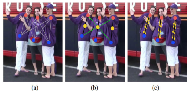
FIGURE 3. Part association strategies. (a) The body part detection candidates (red and blue dots) for two body part types and allconnection candidates (grey lines). (b) The connection results using the midpoint (yellow dots) representation: correct connection (black lines) and incorrect connections (green lines) that also satisfy the incidence constraint. (c) The results using PAFs (yellow arrows). By encoding position and orientation over the support of the limb, PAFs eliminate false associations.
