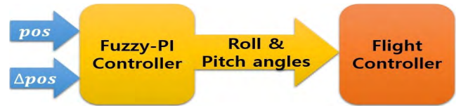
FIGURE 6. Block diagram of the proposed fuzzy logic controller.
