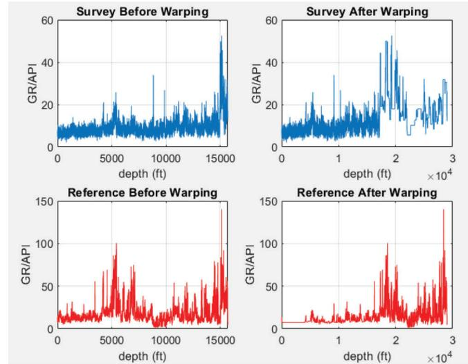
**Fig. 10**—Illustration of overfitting between the survey and the reference logs using DTW.
