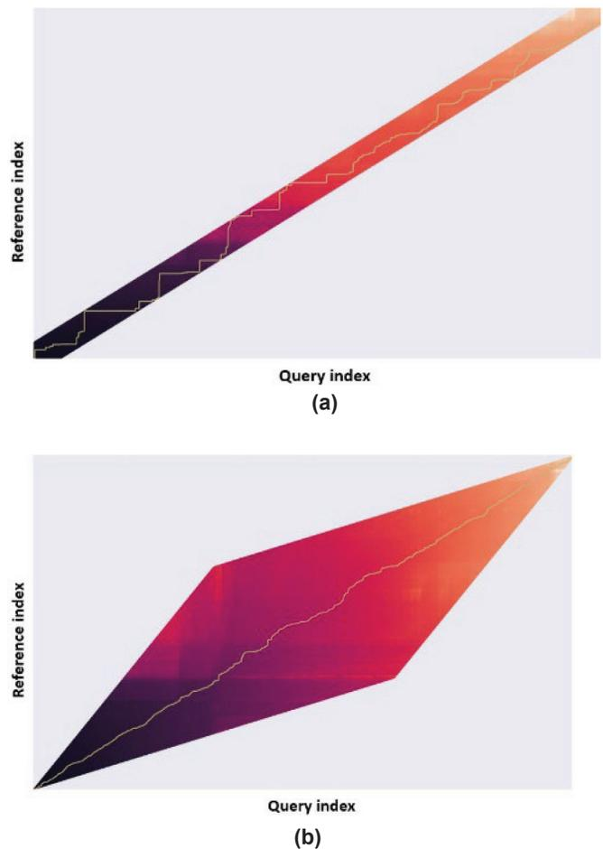
**Fig. 3**—Constrained DTW methods: (a) Sakoe-Chiba and (b) Itakura. Please note the darker the shade, the lower the cost.
