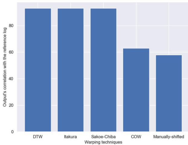
**Fig. 9**—Comparing the highest correlations each method's outputs give with the reference log against that of the manually shifted log.
