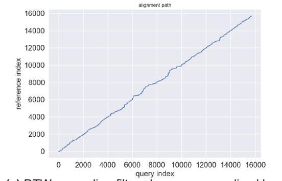
(a) DTW on median-filtered z-score normalized logs
