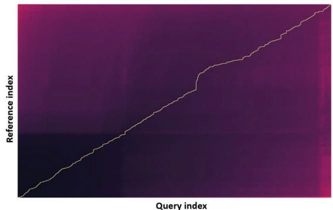
Fig. 2—Alignment path on a global cost matrix. Please note the darker the shade, the lower the cost.
