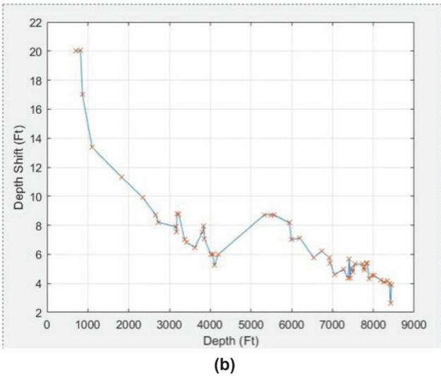
Fig. 7—(a) Alignment paths for the manually shifted depths. (b) Shift profile for the manually shifted depths.
