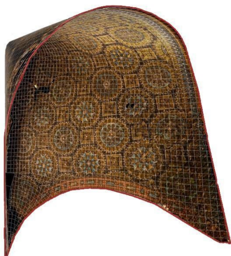
Figure 25. Rendering of the conic vault together with its mesh.
