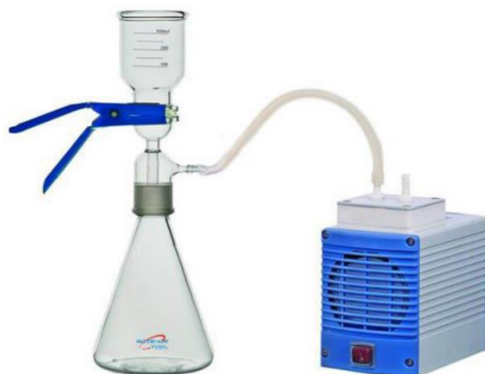
Figure S1. Vacuum filtration device used when AFs are deposited on the separator.
