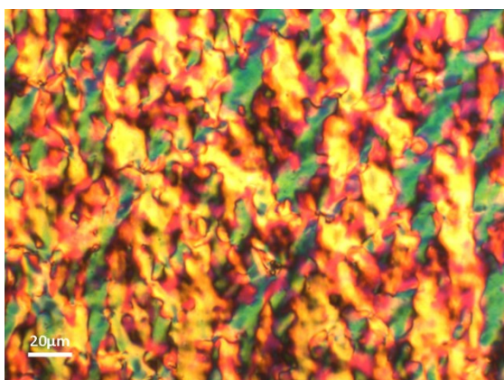
Figure S5. Domains of differing birefringence with boundaries in the N_F phase between untreated glass slides ( T = 51\text{ }^{\circ}\text{C} ).
