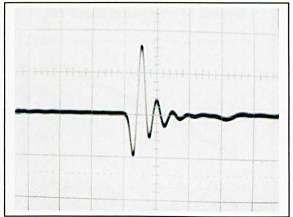
**Figure 2.9(a): Simulated pulse using a 300 point IFFT** **Figure 2.9(b): Measured pulse by practical measurement system. Vertical axis = 0.1V/div**
