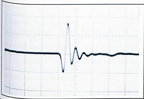
Figure 7(b): Observed pulse waveform Vertical axis = 0.1V/div
