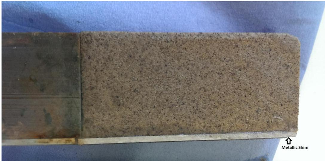
**Figure 5-2. Set metallic shim. Metallic shims were set symmetrically on the plug halves' edges. Note the attachment of flow accumulating cap (Left) to the sandstone plug (right) and use of the shims on the metallic plug as well as the sandstone plug.**
