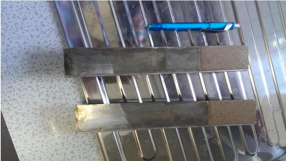
**Figure 5-4. Sandstone half plugs attached to the flow accumulating plugs ready for flooding test.**
