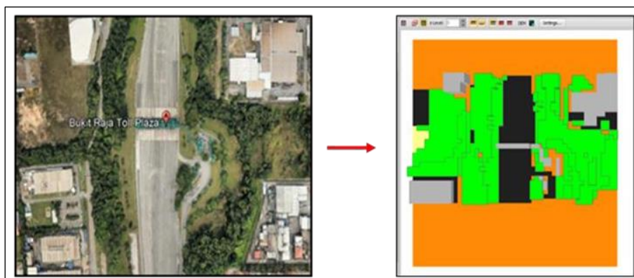
Figure 4. Bukit Raja Toll from Google Earth Image was Modelled Into the SPACE Tool in Envi-MET Software
