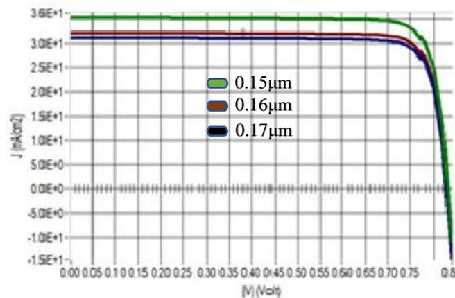
Fig. 4. Influence of absorber thickness on the J-V Characteristic
