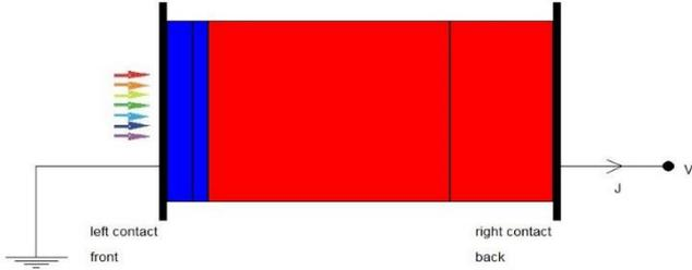
Fig. 2. The heterojunction Structure in SCAPS
