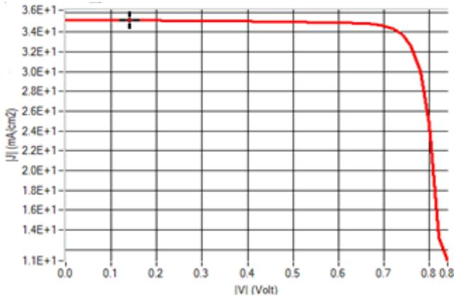
Fig. 3. Optimal J-V Characteristic from the solar cell
