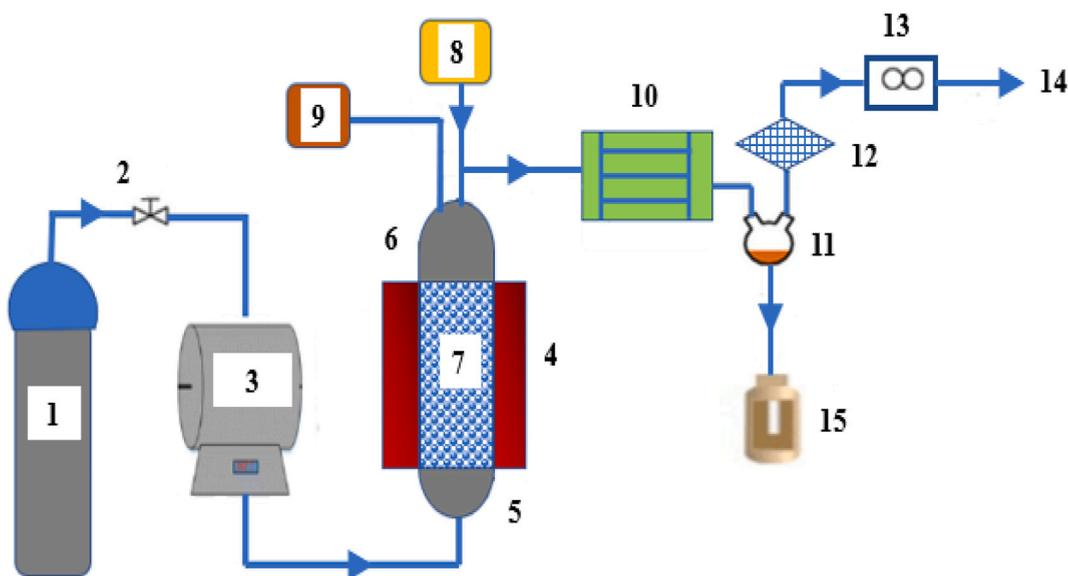
Fig. 1. Set up of the pyrolysis reactor used in the experimental work (1) nitrogen gas tank, (2) flow controller, (3) gas heater, (4) furnace with electrical tubes, (5) char collector, (6) pyrolysis reactor, (7) biomass bed, (8) biomass lock hopper, (9) Thermocouple (10) condenser, (11) condensation & gaseous separator, (12) filter, (13) gas flow meter, (14) gas output (15) extracted bio-oil.
