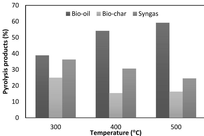
Fig. 2. Effect of different temperatures on the pyrolysis products.
