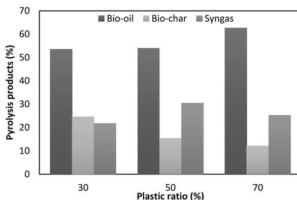
Fig. 3. Effect of different plastic ratios on pyrolysis products.
