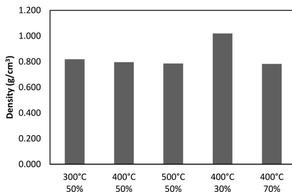
Fig. 4. Effect of different pyrolysis temperatures and plastic waste ratio in the bio-oil density.
