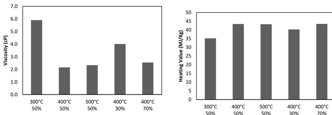
Fig. 5. Effect of different pyrolysis temperatures and plastic waste ratio in the bio-oil (a) viscosity; (b) heating value.
