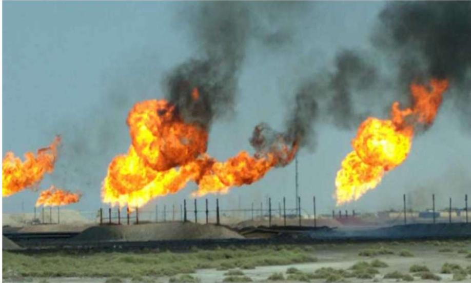
*Figure 5: 3.1: Image of gas being flared during oil and gas production. Source: Modern diplomacy (2018) <https://modern diplomacy.eu/2018/07/18/new-satellite-data-reveals-progress-global-gas-flaring-declined-in-2017/> (accessed 28/08/2020).*
