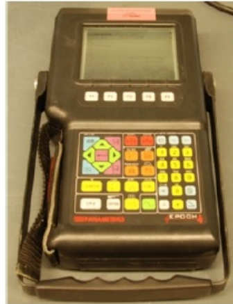
Figure 3.2: Instrument used for measuring the velocities of shear and compressive waves to determine the Poisson's ratio and Young's modulus.
