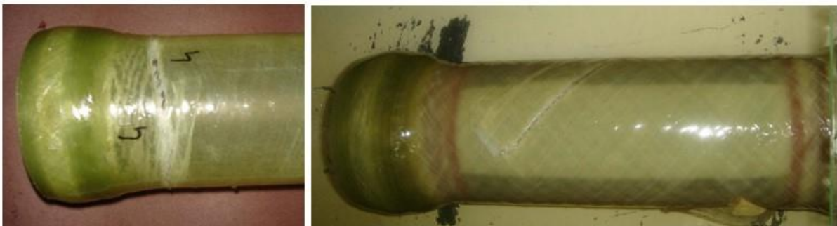
Figure 7: Composite tube after burst failure testing, (Source: [59])
