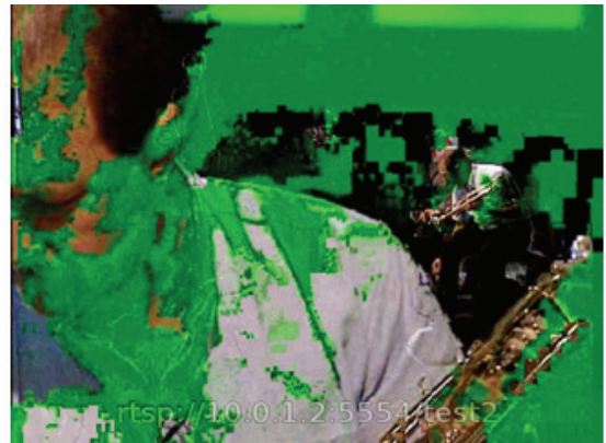
Figure 4. Sample decoded frame obtained streaming Test1 over a network path with capacity 1.5 Mb/s and buffer size of 10 packets.
