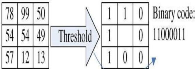
Fig. 3 The basic LBP operator.
