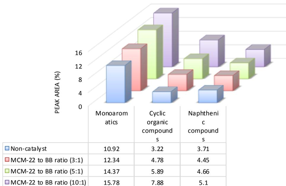
Figure 6: (a) Chemical compounds produced in non-catalytic and catalytic (layered zeolites) fast pyrolysis of *B. braunii* at 550 °C (b) Monoaromatics and naphthenic compounds produced over layered zeolite as a function of catalyst/biomass ratios.
