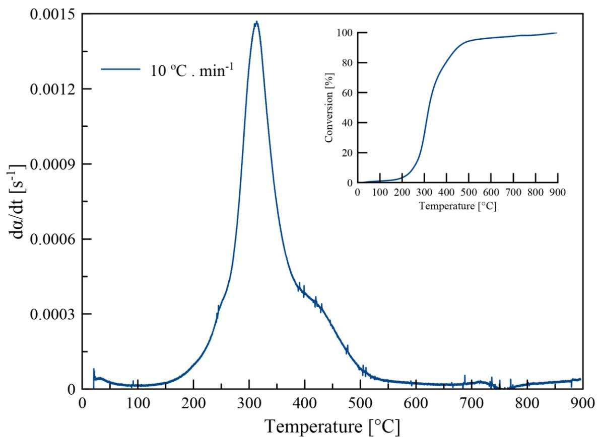
Figure 2: Thermogravimetric mass loss (TG) and differential mass loss (DTG) curves for *B. braunii* at 10 °C/min.
