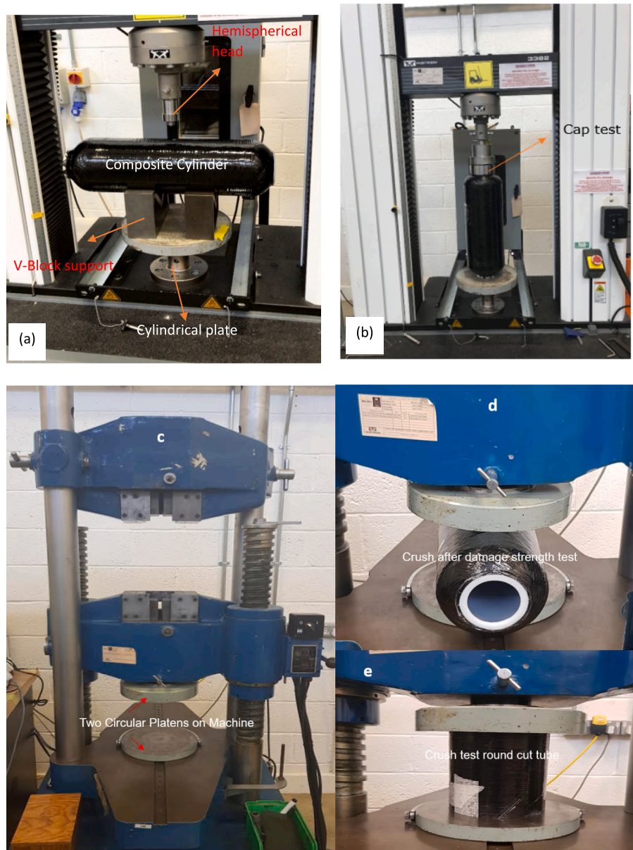
Fig. 2. (a) Instron machine with the vessel ready for compression testing in the transverse (b) in the axial direction (c) Intron-XH03 equipment having a 600 kN load capacity (d) vessel in between two circular platens (e) round cut pressure vessel.
