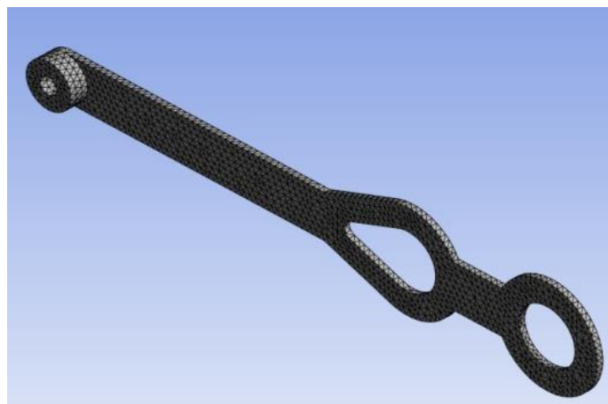
Figure 6. Resistance Band Analysis Mesh Example of t=1mm, Lo=50mm, F=5.
