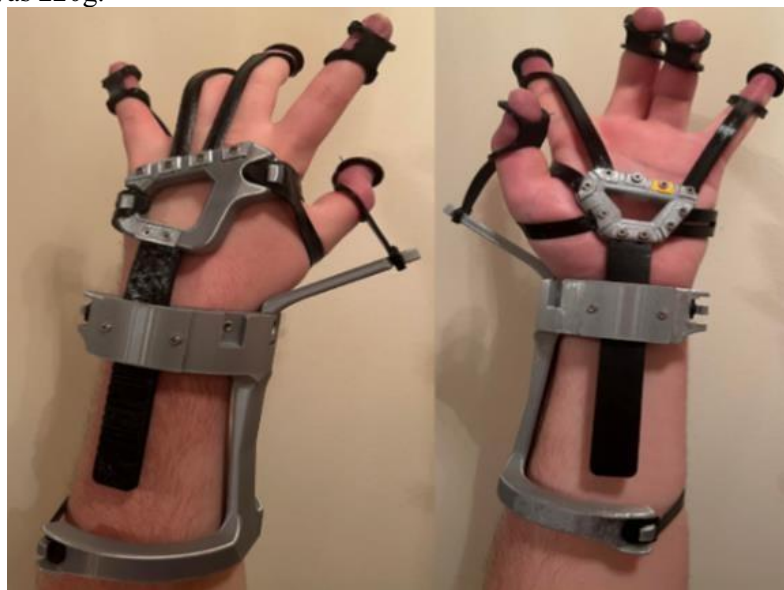
Figure 5. Final assembled burn rehabilitation brace worn in multiple views
