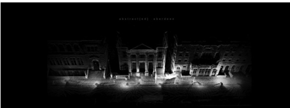
Figure 2. Point cloud image of the theatre building in xxxxxx (author owned, 2020).
