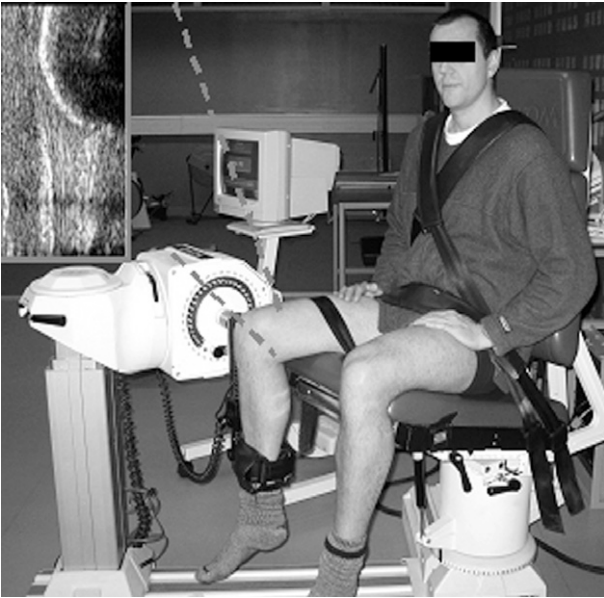
Fig. 2. Experimental set-up. Isometric knee extension torque was determined by fixing the knee at 90° flexion (full extension = 0°) and hip at 85° (supine = 0°). The knee joint centre was aligned with the centre of rotation of the dynamometer lever arm and straps were fixed across the chest, hip and thigh of the test limb to prevent any extraneous movement. A padded cuff was strapped on the lower leg at ~3 cm above the medial malleolus. Inset - showing sagittal plane ultrasound image of patellar and tendon.
