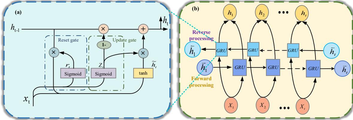
Figure 1. Improved RNN structure diagram. (a) GRU single-celled structure. (b) BiGRU.
