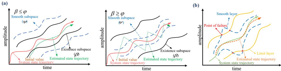
Figure 2. Improved SVSF algorithm. (a) SSVSF algorithm principle diagram. (b) TSVSF algorithm principle diagram.
