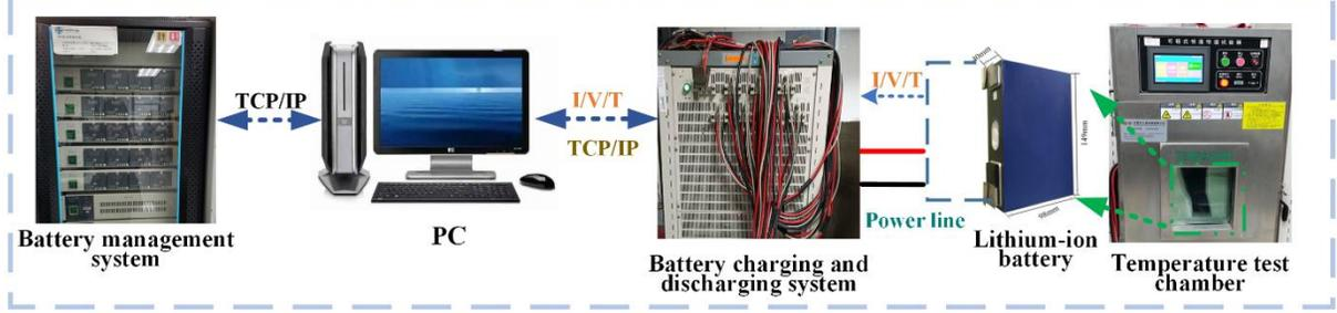
Figure 4. Lithium-ion battery test platform
