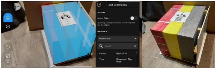
Figure 10. Prototype model (left). Prototype BIM Model overlaid in AR (right).
