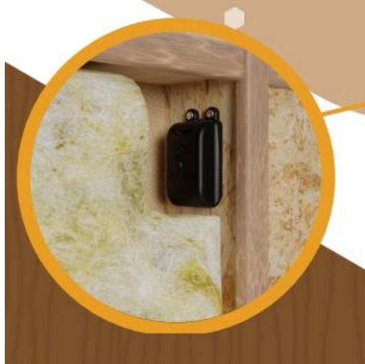
Figure 2. Example of measuring with a insertion moisture meter from Woodsense
