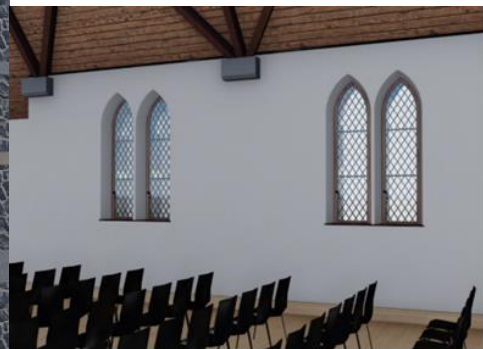
Figure 15. Render of the Replica Clear Glass Window from inside the Columban Hall (Source: Author).
