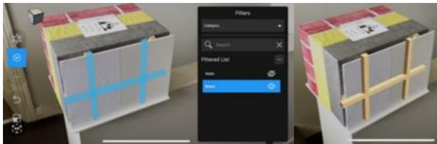
Figure 15. Visualisation of concealed battens with AR
