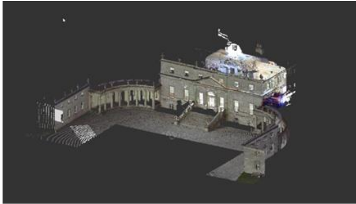
Figure 4. Fully Registered Point Cloud External and Internal
