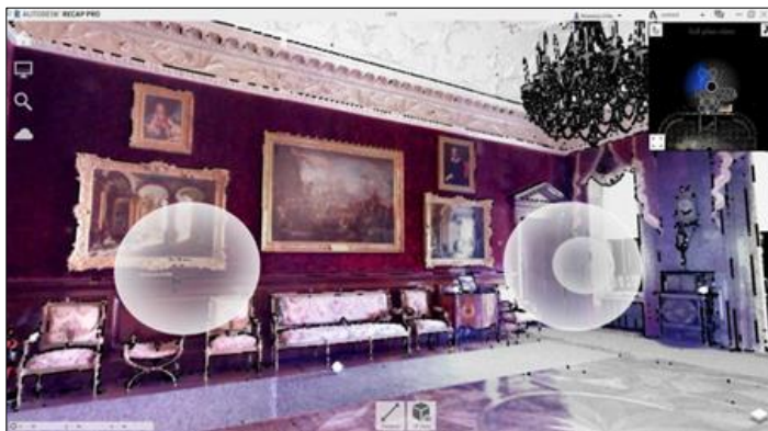
Figure 2. Position of spheres showing scan positions
