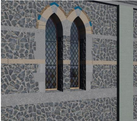
Figure 16. Render of the Replica Window with Stained Glass (Source: Author).
