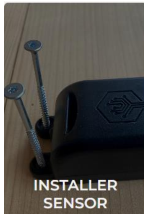
Figure 6. Woodsensor with the screws that are measuring humidity by resistance - by Woodsence.
