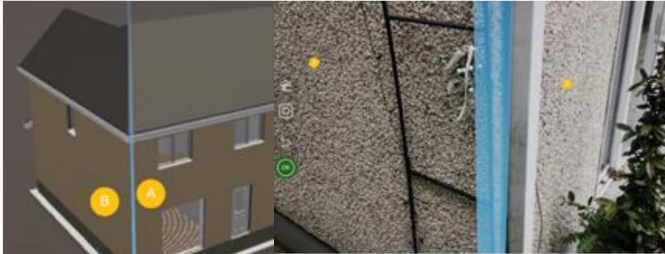
Figure 14. Example of corner alignment of BIM model into real world AR visualisation
