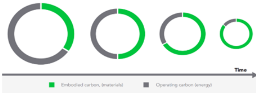
Figure 1. The importance of embodied carbon (materials) grows as operational energy decarbonizes.
