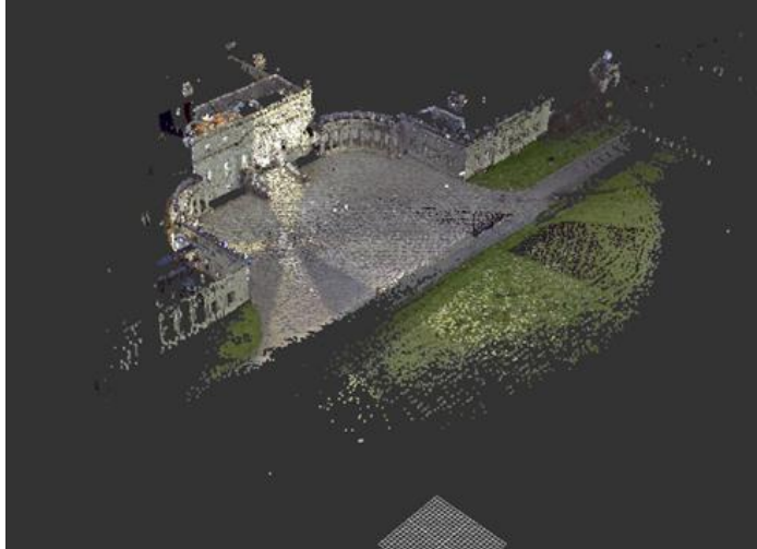
Figure 5. Isolating Parts of the Point Cloud in ReCap.
