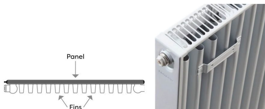
Figure 1. Type 11 domestic panel convector.
