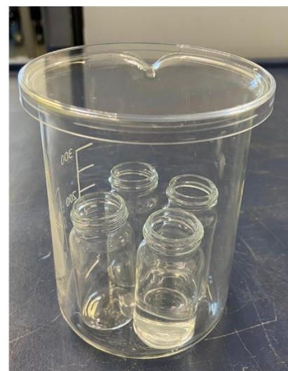
Figure 5.6: Adapted incubator used for each treatment consisting of four 20 mL vials grouped in a 400 mL beaker covered with a polystyrene petri dish.
