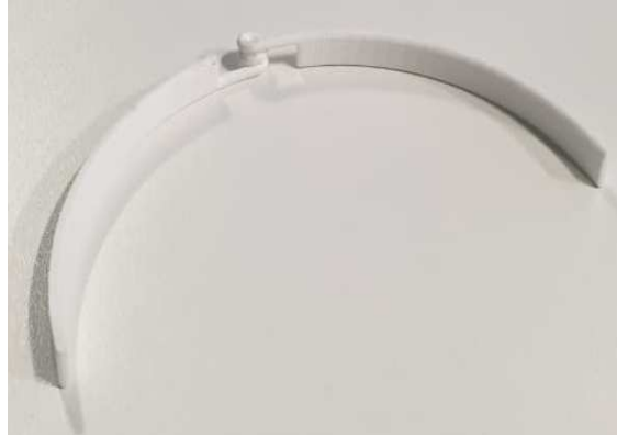
Figure 3.5: 3D printing of torsion spring snap-latch ring (6 ring module, Prototype II), showing various views, at full made of Acrylonitrile-Butadiene-Styrene (manufactured using the INTAMSYS FUNMAT PRO HT 3D printer at School of Engineering in Robert Gordon University (CAD model in Appendix I)
