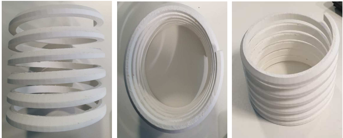
Figure 3.4: 3D printing of spiral Snap-Latch Ring design (6 ring module), showing various views, at full made of Acrylonitrile-Butadiene-Styrene (manufactured using the INTAMSYS FUNMAT PRO HT 3D printer at School of Engineering in Robert Gordon University).
