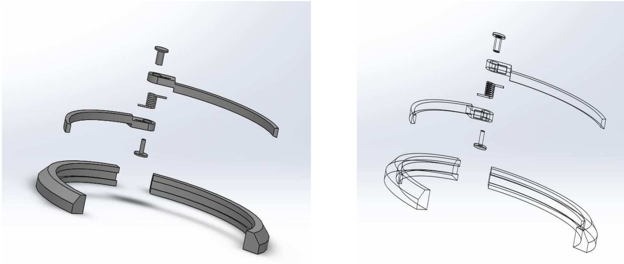
Figure 5.4: Exploded view of Prototype II (showing all the seven components).
