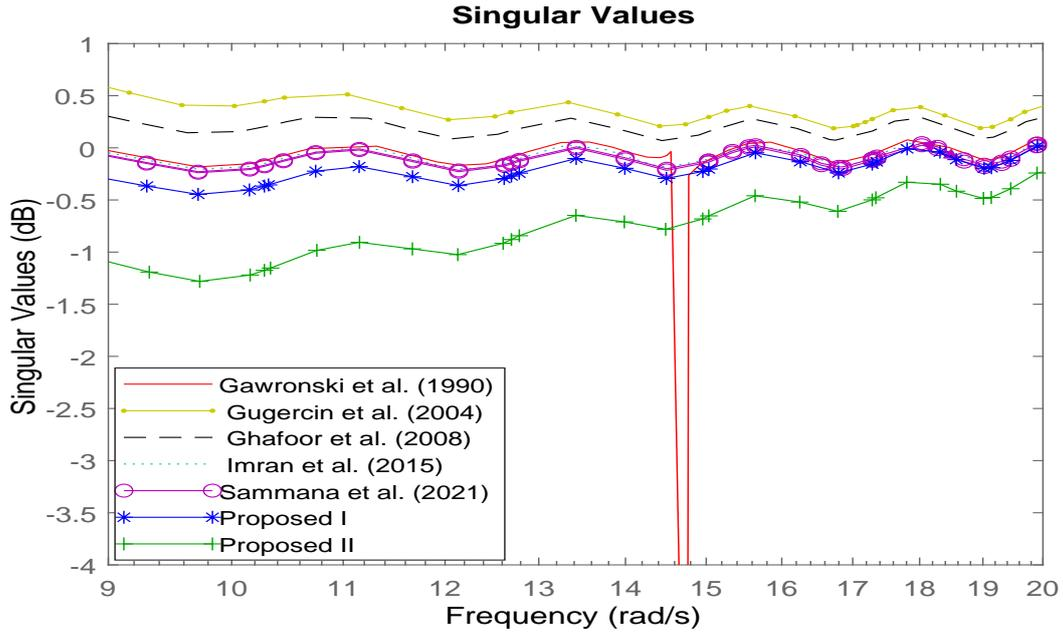
Figure 4. Close-up view of  $\sigma[G_{50}(s) - G_3(s)]$  in  $[\omega_1, \omega_2] = [9, 20]$
