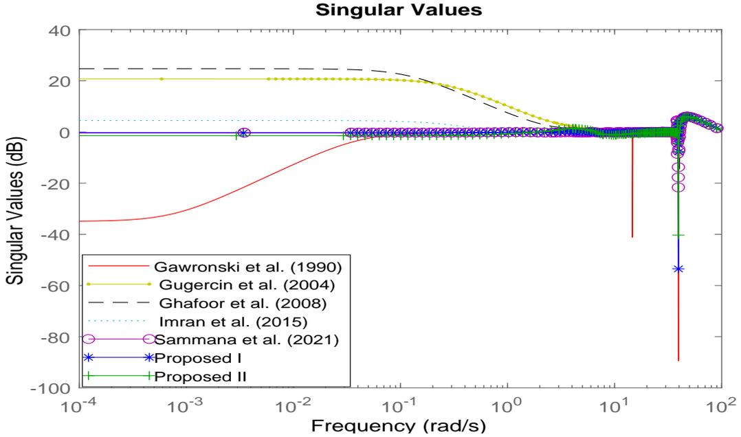
Figure 3. Frequency response error comparison  $\sigma[G_{50}(s) - G_3(s)]$
