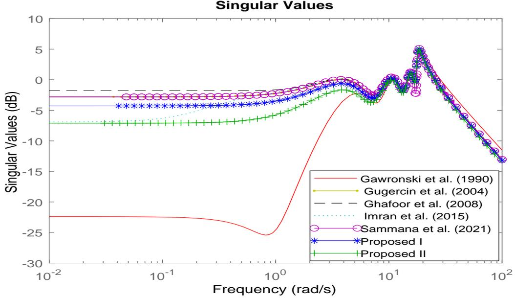
**Figure 1.** Frequency reponse error comparison  $\sigma[G_8(s) - G_1(s)]$
