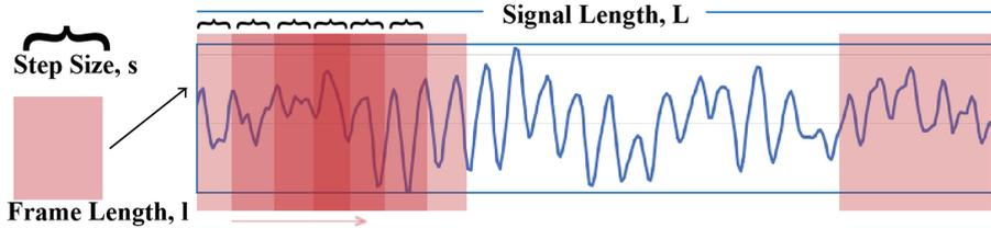
Fig. 1. Skimming frame process for generating samples.
