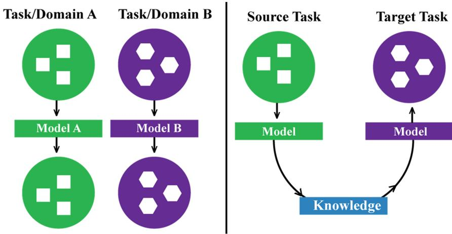
**Fig. 3.** (a) A traditional machine learning approach is presented which has two independent models for two different tasks; (b) a transfer learning approach is shown where the two tasks are denoted as source task and target task and knowledge is transferred between the tasks.
