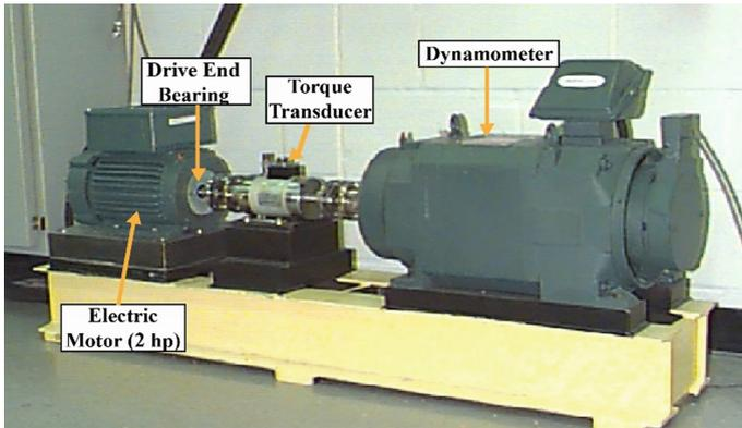
Fig. 6. Experimental set up by Case Western Reserve University [12].
