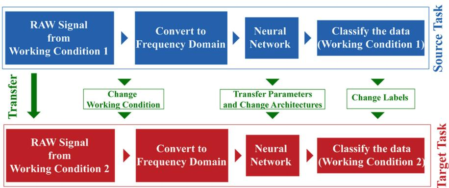
**Fig. 5.** Block diagram of the proposed model.
