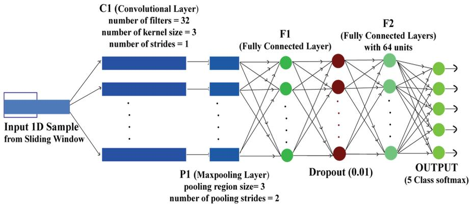
Fig. 4. Detail architecture of 1D CNN.
