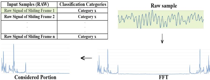
Fig. 2. FFT process for preprocessing the RAW signal.
