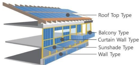
Figure 2. BIPV integration in buildings [26].
