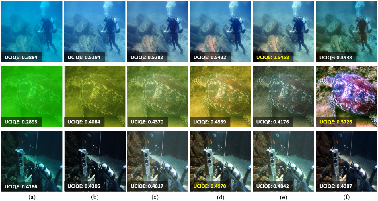
Figure 5: Three sample raw underwater images (a) and their enhanced versions (b)-(f) produced by different variations of the DICAM model, i.e (b) without the CAM modules, (c) without the color correction stage, (d) original DICAM with 60 epochs, (e) original DICAM with 120 epochs, and (f) the reference image.
