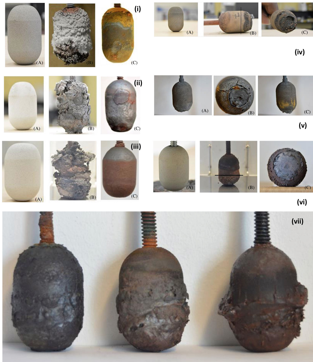
FIGURE 7 Examples of immersion tests in Cu—Cl: (i) SHS-9172 specimen; (A) before, (B) after, and (C) after cleaning, (ii) SHS 9172 + \text{Al}_2\text{O}_3 specimen; (A) before, (B) after, and (C) after cleaning, (iii) SHS-9172 + YSZ specimen; (A) before, (b) after, and (c) after cleaning, (iv) Diamalloy 4006 sample (100 hr test); (A) before, (B) after, and (C) after cleaning, (V) Diamalloy 4006 + \text{Al}_2\text{O}_3 specimen (100 hr test); (A) after, (b) sample tip after, and (c) specimen with green shades after, (vi) Diamalloy 4006 + YSZ specimen (100 hr test); (A) before, (B) after, (C) sample tip after, and (vii) Diamalloy 4006 + YSZ, Diamalloy 4006 + \text{Al}_2\text{O}_3 , Diamalloy 4006 specimen (left to right) after the immersion test for 50 hrs (scale bar not available) 58 (Source: permission obtained ©M.S. Azhar, all rights reserved).
