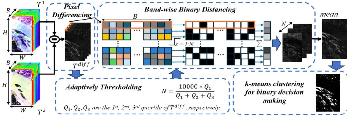
Fig. 1. Architecture of the proposed ABBD algorithm.
