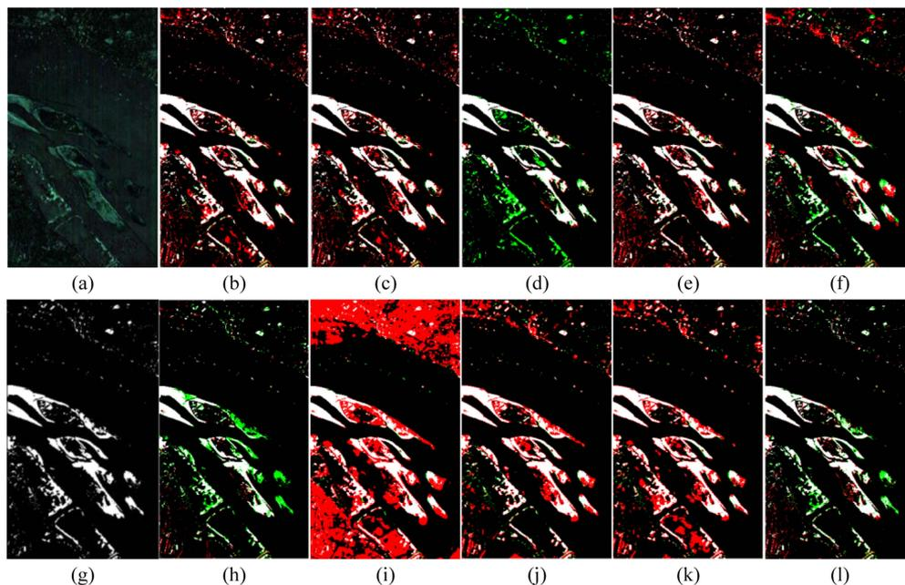
Fig. 5. Extracted change maps on the River dataset from different methods of (b) AD; (c) CVA; (d) SAM; (e) PCA; (f) IR-MAD; (h) DTW-KM; (i) PTCD; (j) TDRD; (k) SALA and (l) our ABBD in comparison to the pseudocolor image of the difference between (a) bitemporal images and (g) the ground-truth map, where the false alarms and missing pixels are labeled in red and green, respectively.
