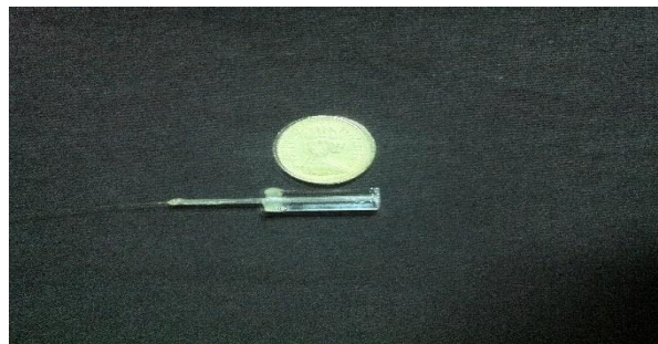
Figure 4.12 Fabricated multiplexed FBG/EFPI sensor head (The sensing head placed close to a pound coin to show the small size)
