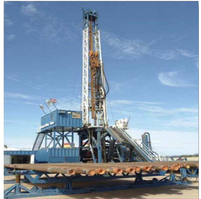
Fig. 9 Casing drilling rig [31]
